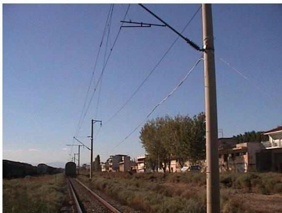
Sensor cable mounted between two pylons at Thessaloniki-Aghialou
